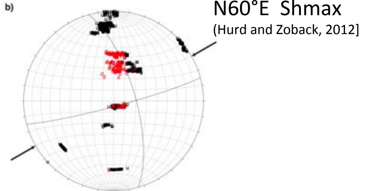
**If double-couple, plane of seismicity is right-lateral – contrary to stress. More likely that first motions reflect combined tensile & shear failure.**
