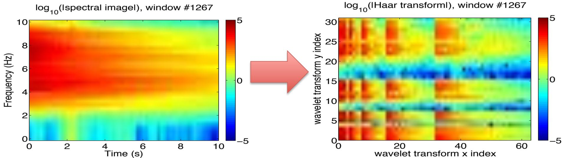
Goal: compress nonstationary seismic signal
