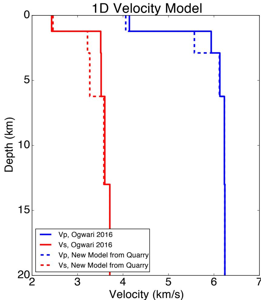
**Improved  $P$  and  $S$ -wave velocity structure based on known quarry blasts using Velest.**
