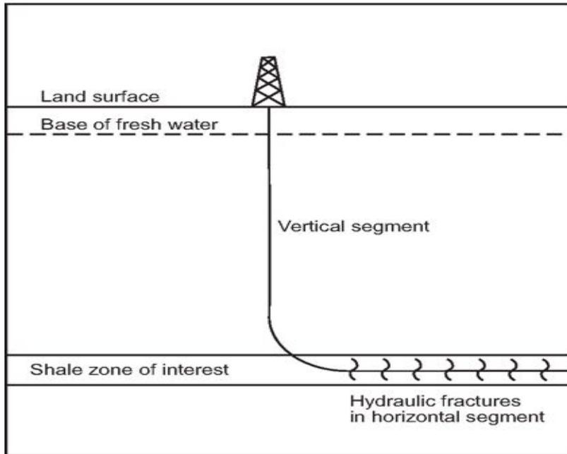
Hydraulic Stimulation (Fracking) wells use a staged injection of fluid to increase permeability and access hydrocarbons.
