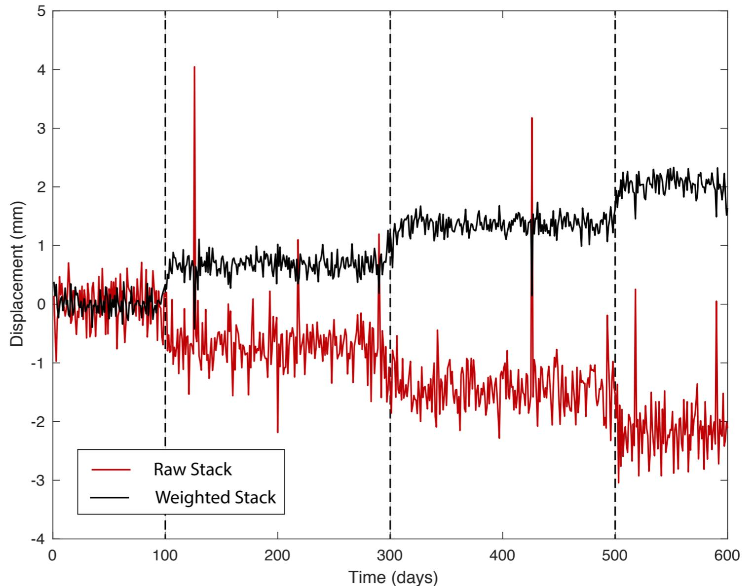
Sum of the GPS time series, **weighted by the amplitude of the synthetic template**
