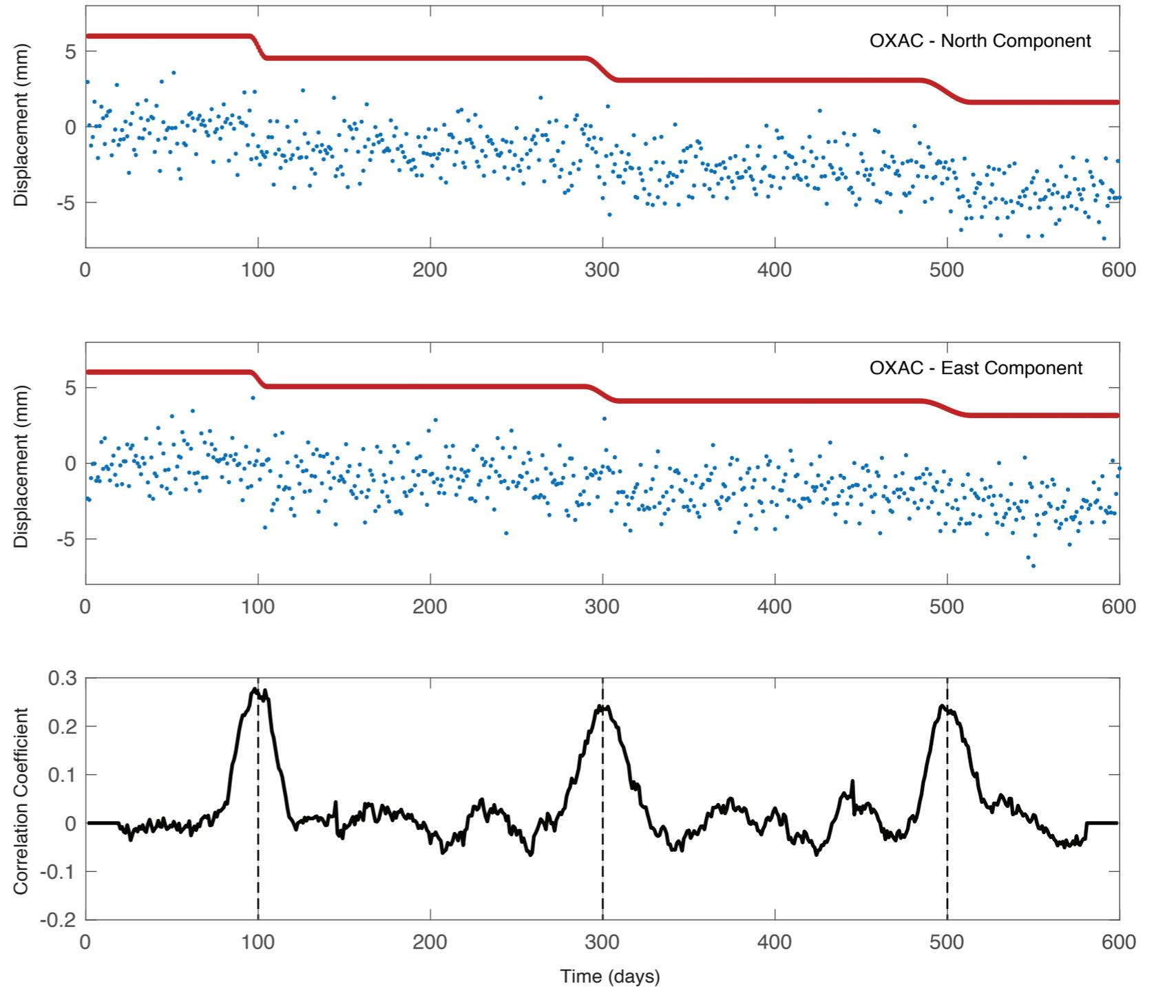
Normalised correlation function, stacked over the East and North time series, and **weighted by the amplitude of the synthetic template**
